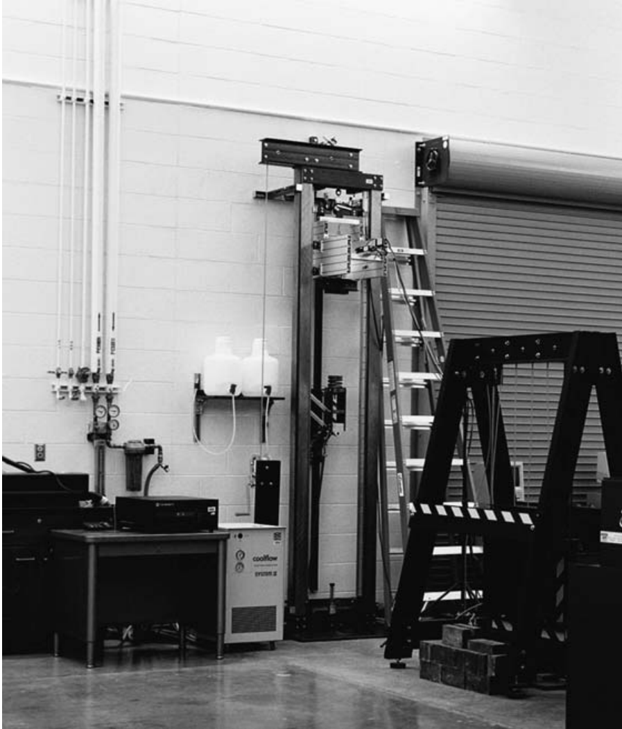
FIGURE 1. The 3 m drop tower with the sled positioned at the top of the rails.
