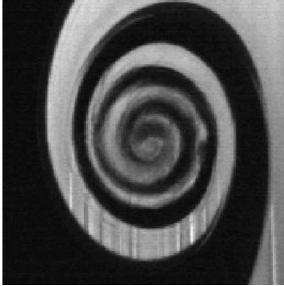
FIGURE 24. Close-up of a vortex core during the early stages of the secondary instability.
